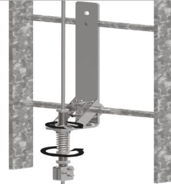
Use adjustable wrenches to hold the integral nut on the top of the threaded shaft whilst tightening the upper M20 nut on the threaded shaft. The upper M20 nut pull against the bottom anchor bracket and start to introduce tension into the cable. Once the system pre-tension has been completed cut off the surplus cable leaving 1-2" and affix the vinyl protective cap.
