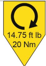
Evenly tighten the nuts to a torque of 14.75 ft lb (20 Nm).
