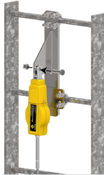
Secure the absorber onto the top anchor by the bolt and castellated nut provided with the absorber. Use the 19 mm wrench to rotate the nut until the split pin can be inserted through the hole in the bolt.
