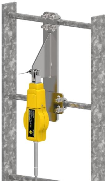
Insert the split pin through the castellated nut and bolt. Split the ends of the pin to ensure the nut is captivated on the bolt.
