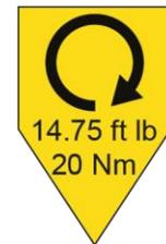
Evenly tighten the nuts to a torque of 14.75 ft lb (20 Nm).
