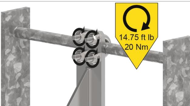
Evenly tighten the nuts using the deep socket to a torque of 14.75 ft lb (20 Nm).
